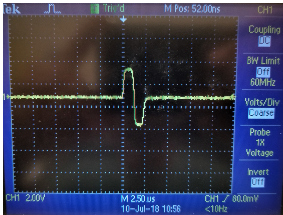
Figure 6. A photograph of the output pulse from the TAC on the second oscilloscope. The amplitude of this pulse reflects the decay rate of the positronium.
